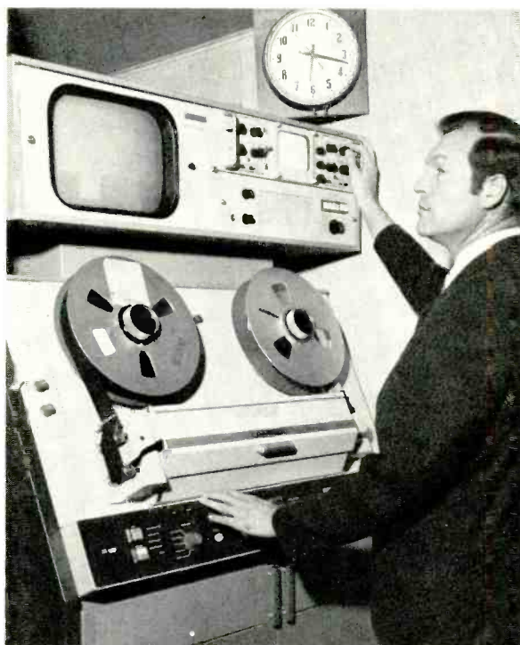
Fig. 3 The conversion from black and white to color mobile facilities was supervised by Ned May, WWJ-TV facilities supervisor. Here he tries the unit's VR 1200B videotape machine.
